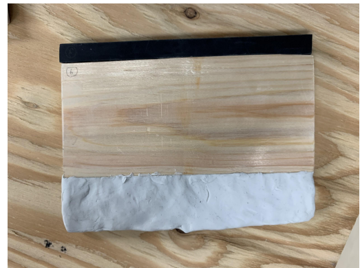
pic.2 ②Attach a piece of rubber 1 cm thick.
